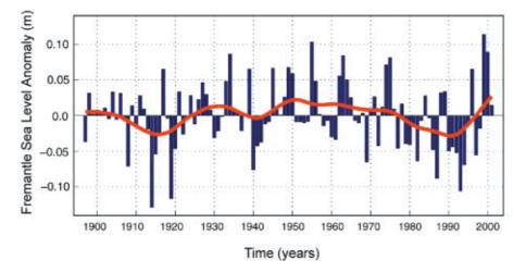
Figure 2: Time series of Fremantle sea level anomaly (variations of annual mean levels from the trend line of Figure 1) shown in blue. The red line shows the interannual variability (El Nino driven) in the record after removing the long-term tidal effects.
