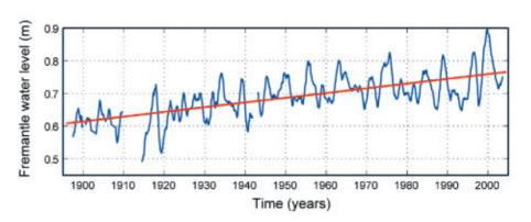
Figure 1: Time series of Fremantle sea level (one year running mean) with the linear trend of 1.54 mm per annum superimposed in red.
