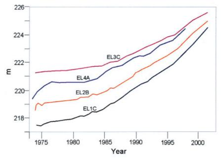
Figure 3: Response of groundwater levels at typical boreholes in the Parmelia aquifer, northern Perth Basin, to replacement of native vegetation by cereals and pasture. The rate of water level rise has accelerated over 30 years.
